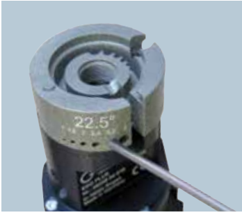
Grinding electrodes: 4 different angles and 6 different electrode sizes
