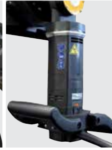
Powerful drive with electronic overload protection and ergonomically designed motor handle
