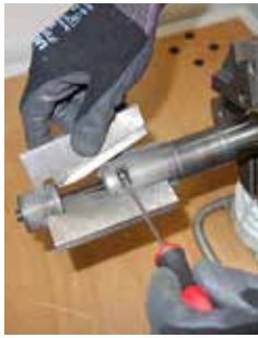
Fast adjustment of the pipe dimension
